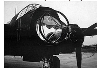
The searchlight installation exposed
